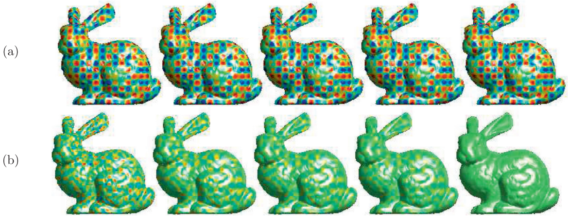
Fig. 6. Convergence of numerical results with refined temporal grids. The results, from left to right, were obtained with \Delta t = 1.563\text{E}-3 , 7.813\text{E}-4 , 3.906\text{E}-4 , 1.953\text{E}-4 , and \Delta t = 2.441\text{E}-5 . (a) Plots of \phi at time T = 0.0125 . (b) Plots of the difference between that grid and the reference solution cell, i.e., \phi - \phi^{\text{ref}} at time T = 0.0125 .
