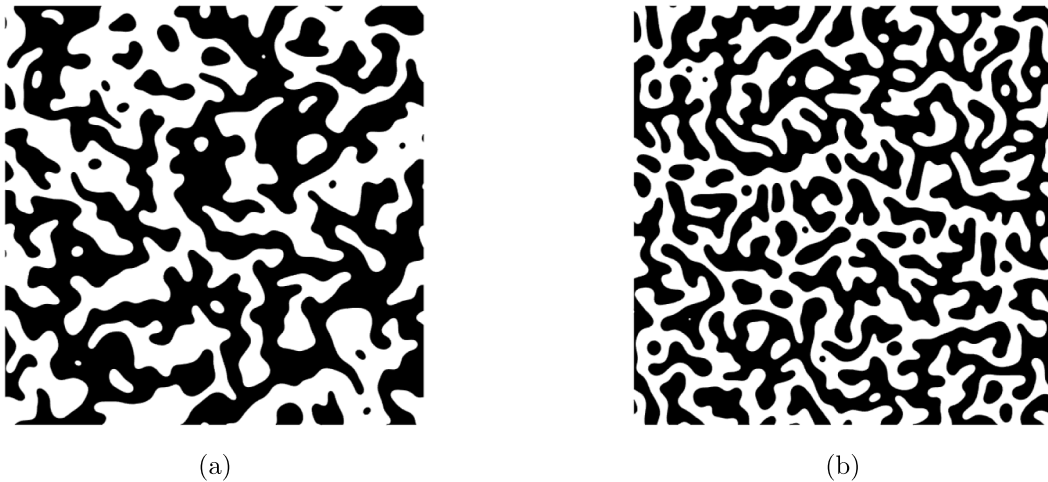
Fig. 1. Snapshots of phase separation by (a) the AC and (b) the CH equations.
