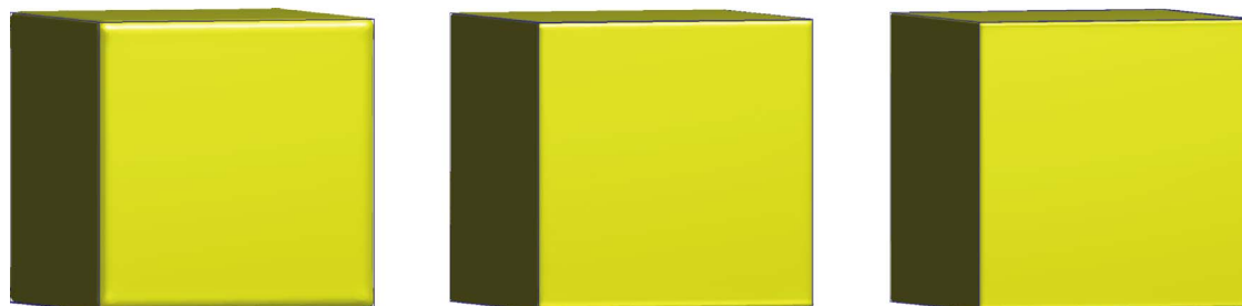
Fig. 3. Recovering sharp features for a cube surface. From left to right, they are reconstructed surfaces using l_2 -norm minimization, l_1 -norm minimization, and our proposed method, respectively.
