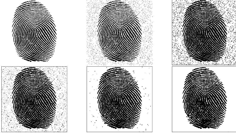
FIGURE 3.2. Finger print. From left to right: (The first row : Initial image, 10% salt-and-pepper noise is superposed over the original, contour of the initial image with noise, The second row : t = 4E-6 , t = 8E-6 , t = 2E-5 ).
