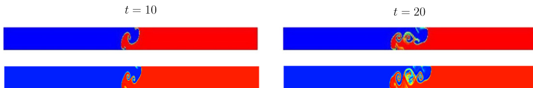
Fig. 3. Comparison with lattice Boltzmann results. Bottom: phase-field obtained by a phase-field method for a channel of aspect ratio 1 : 40. The remaining parameter values are \rho_1/\rho_2 = 1.2 , \theta = 60^\circ , Re = 558.6 , and We = \infty . The heavier and lighter fluids are shown in red and blue, respectively. (For interpretation of the references to colour in this figure legend, the reader is referred to the web version of this article.)
