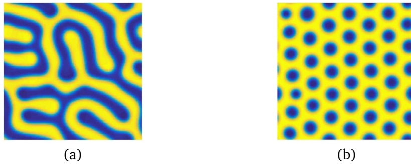
Figure 7: (a) and (b) are the snapshots of the results of diblock copolymer simulation with random initial condition around \bar{\phi} = 0 and \bar{\phi} = 0.3 , respectively. Adapted from [14] with permission of Elsevier Science.
