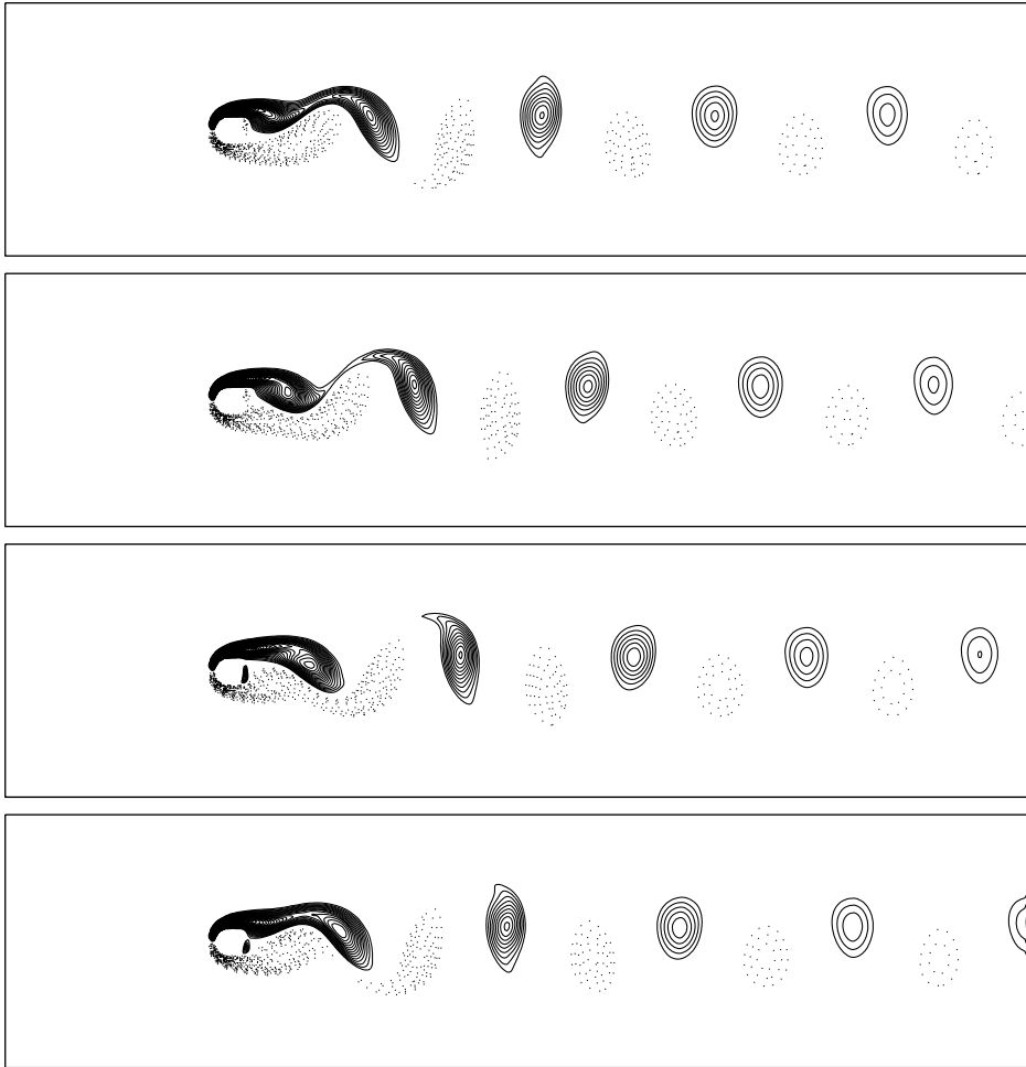
Fig. 2. A cycle of vorticity plots past a circular cylinder at Re = 100 ; solid and dotted lines denote negative and positive levels, respectively.
